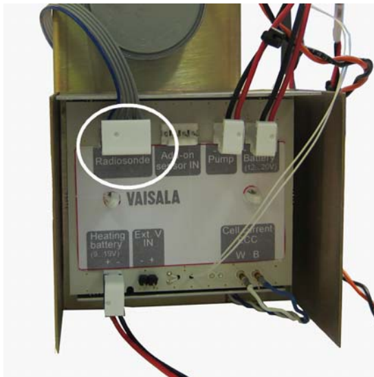
Figure 38 Connecting Radiosonde Cable
