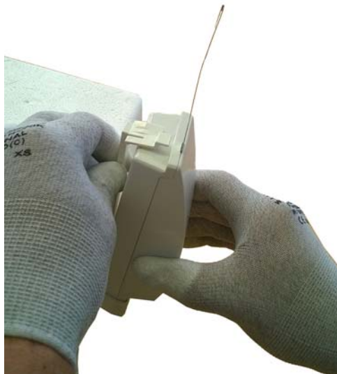
Figure 42 Attaching Radiosonde to the Holder
