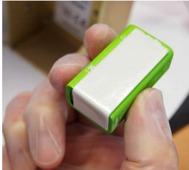
Figure 32 Two-Sided Tape Attached to the Battery
