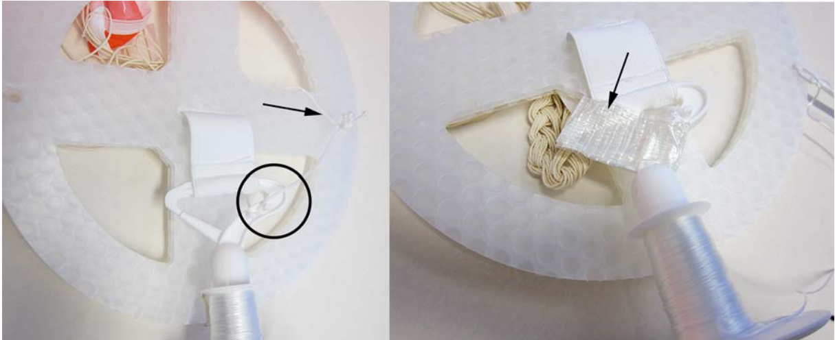
Figure 51 Securing Unwinder with String (Left) or Tape (Right)
