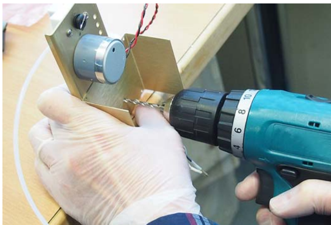
Figure 23 Drilling the Ozone Sensor Frame Holes
