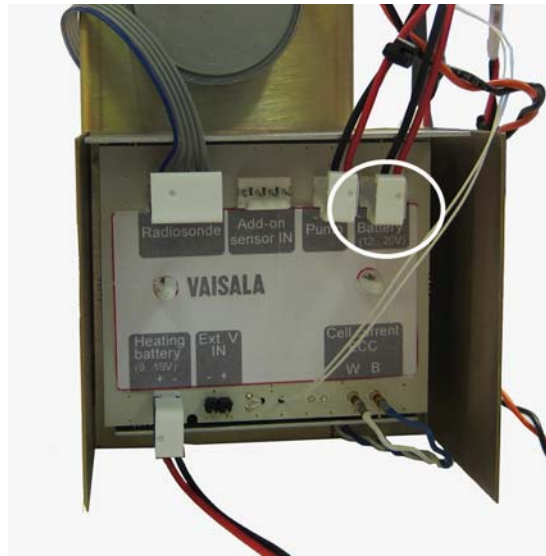
Figure 28 Connecting Ozone Sensor Battery Cable
