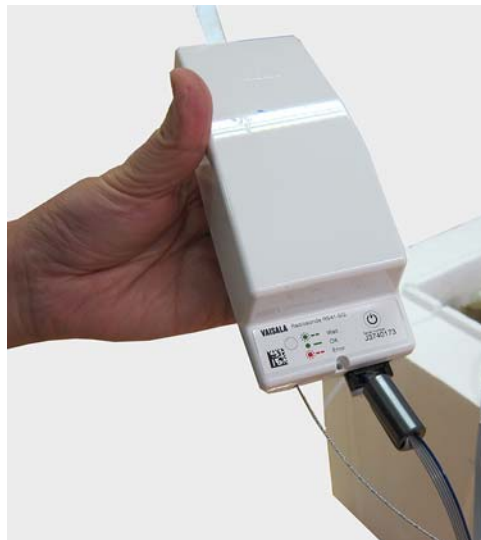
Figure 40 OIF411 Connected to Radiosonde Interface Connector
