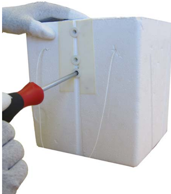
Figure 17 Inserting the Dowels
