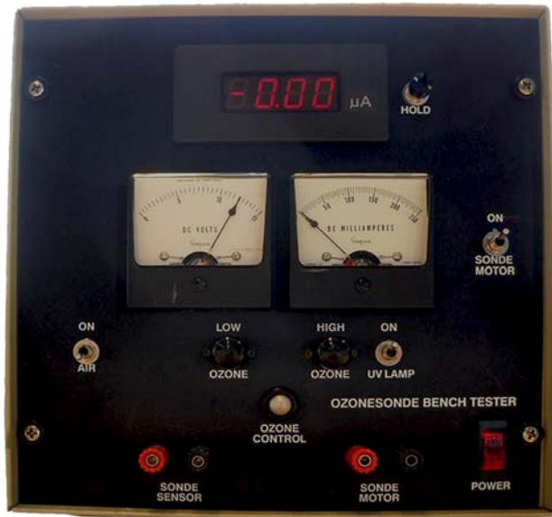
Figure 9 EC Black Bench O3S Tester Made by EC
